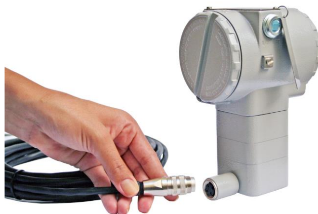
Figure 1.15 - Connecting the Cable to the Position Transmitter
