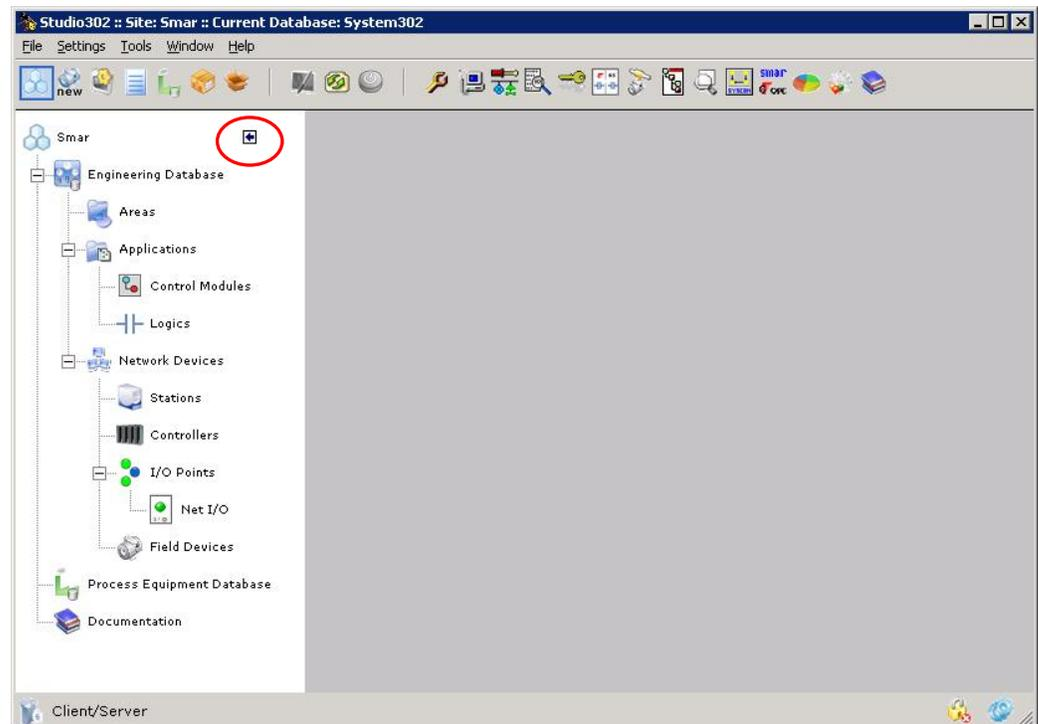
**Figure 2.16. Hiding the topology tree**
