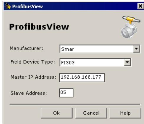
Figure 4.54. Detecting Profibus Devices
