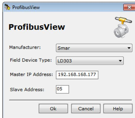
Figure 8.8. Opening the Profibus View dialog box
