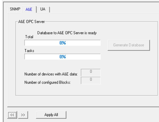
**Figure A.28. Generating initial database for A&E OPC Server**
