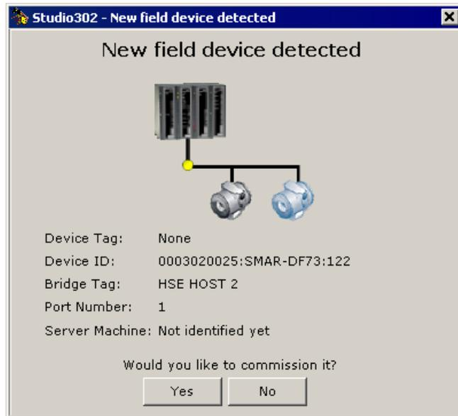
Figure 4.50. Detecting Devices
