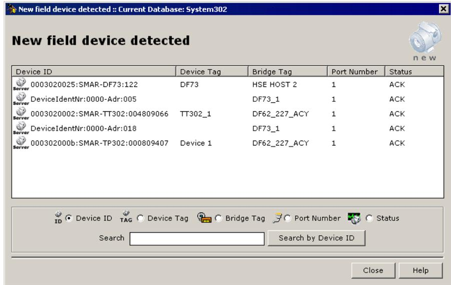
Figure 2.3. New field device detected window
