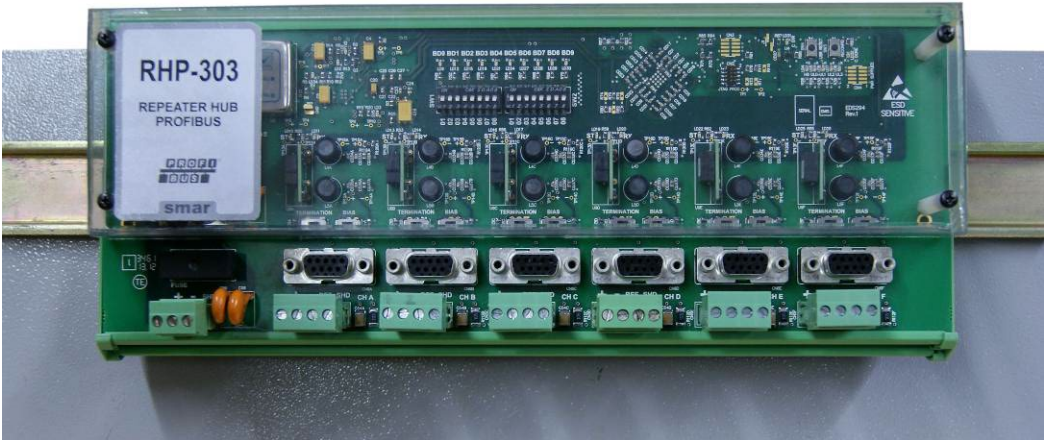
Figure 11 – RHP303 installed on a DIN rail
