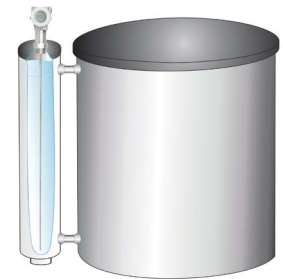
Installation in Communicating Vessel
