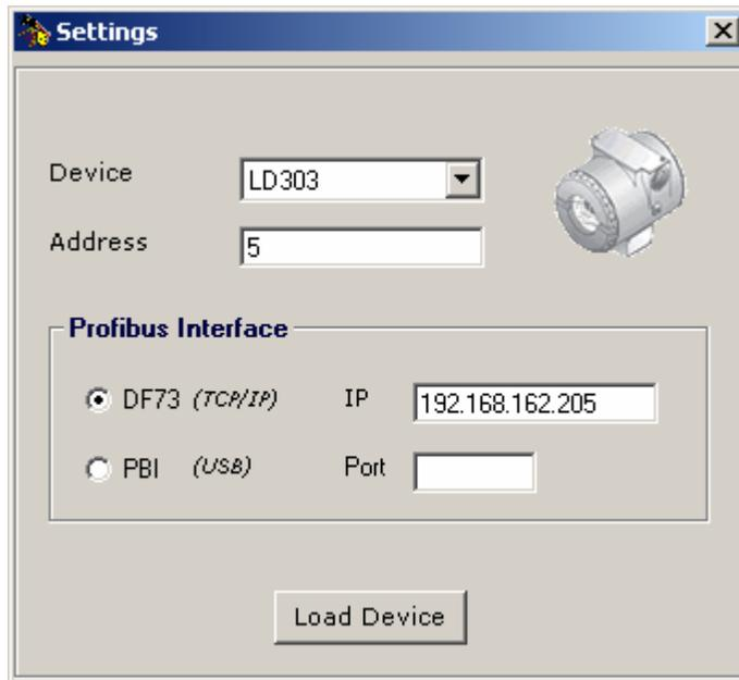
Figure 2 - Setting the Device in Manual Mode
