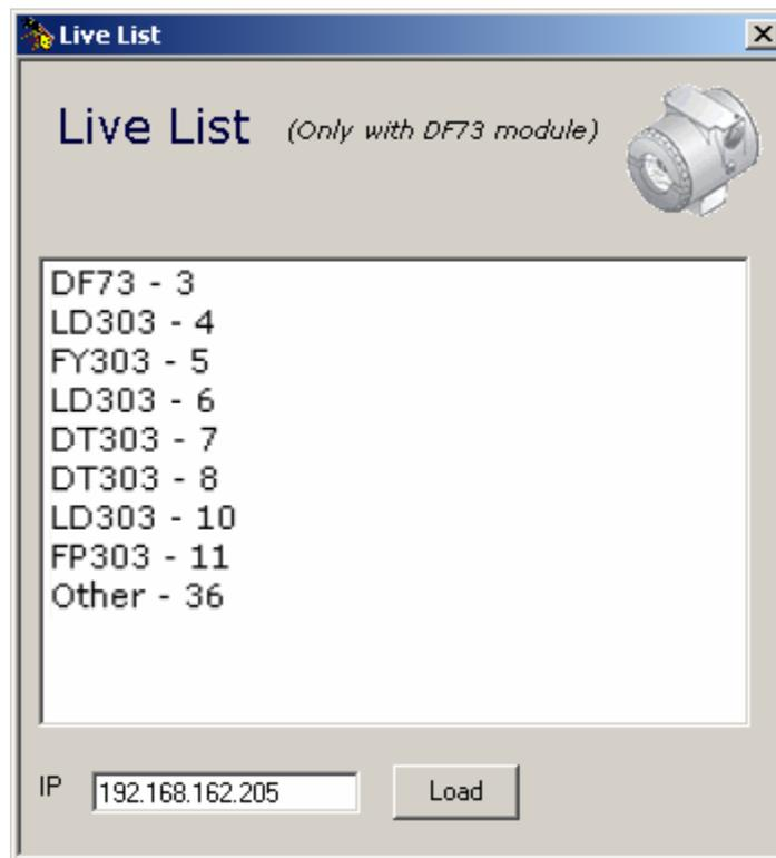
Figure 1 - Live List of the Profibus View Configurator
