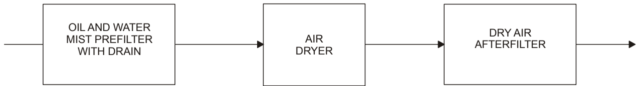
Figure 1.5 – Air Quality Conditioning System
