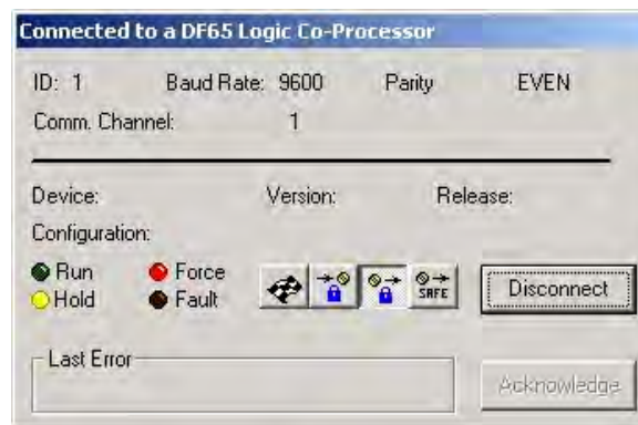
Fig 3.81- LOGICVIEW Connected to the DF65
