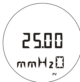
Figure 2.7 – Typical Monitoring Mode Display Showing PV, in this case 25.00 mmH 2 O
