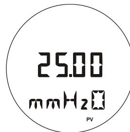
Figure 2.7 – Typical Monitoring Mode Display Showing PV, in this case 25.00 mmH 2 O
