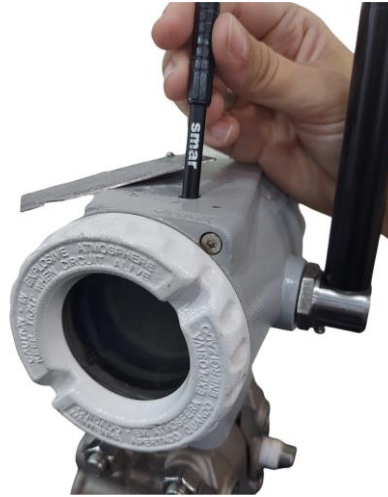
Figure 4.2 – Zero and Span Local Adjustment
