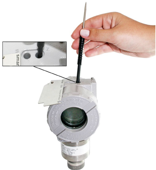
Figure 3.15 - Local Adjustment Holes
