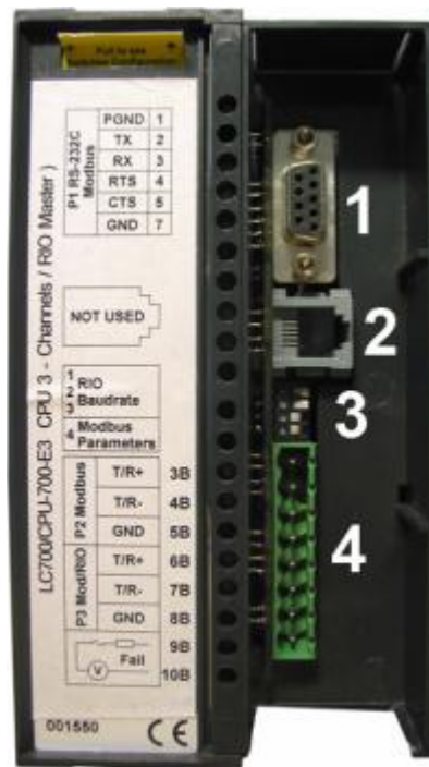
Figure 3.13 - Communication Channels of The CPU-700-E3.
