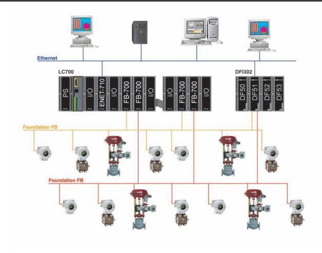
LC700 and DFI302 are sharing the Ethernet line (hub/switch are not showing). A Foundation Fieldbus configuration can be sent to any of the Fieldbus networks from the PC. The configuration from the PC will pass through the DFI302 and search the field devices.
