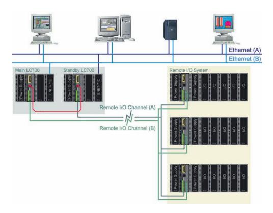
Redundant system with double Ethernet (hubs/switches are not shown), double Remote I/O lines and double Power Supplies on every Remote I/O system.
