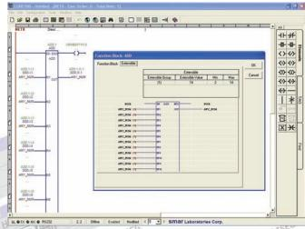
Function Blocks with configurable number of inputs
