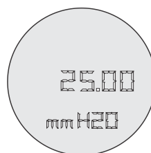
Figure 2.3 – Typical Monitoring Mode displaying the 25,00 mmH 2 O value
