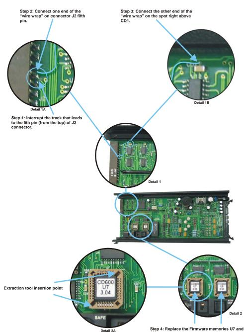
Remove the memory chips from the socket.
