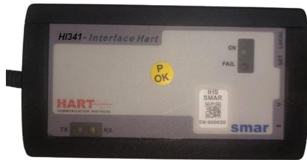
Figure 16 – – Indication of the NET/LOCAL and I/V selector switches
