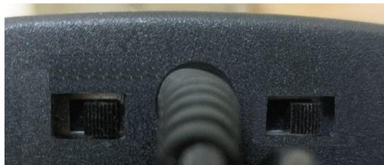
Figure 17 – Detail of the NET/LOCAL and I/V selector switches
