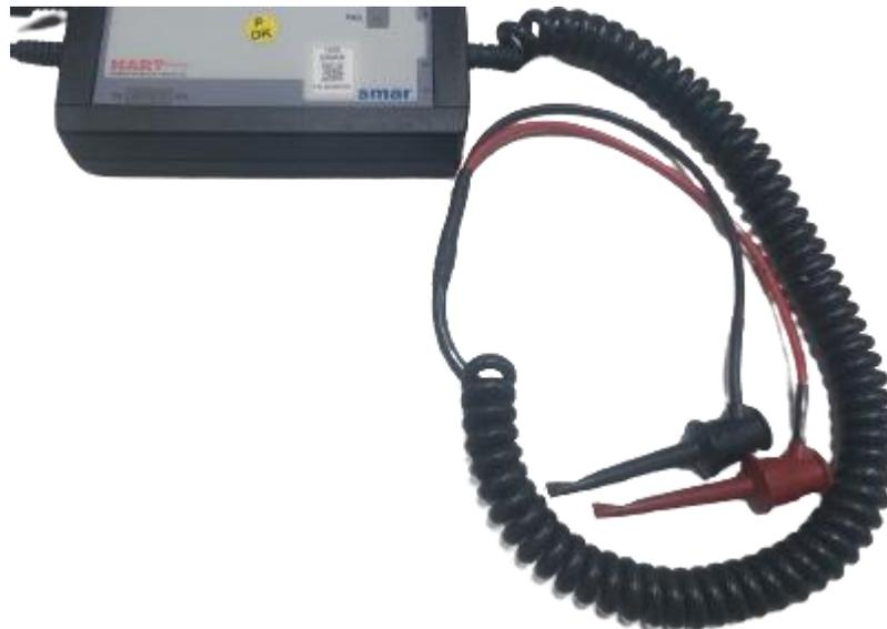
**Figure 12 – Retractable hooks for connection to HART equipment**
