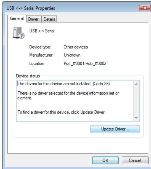
**Figure 7 – Driver Installation Step-by-Step – Update Driver**
