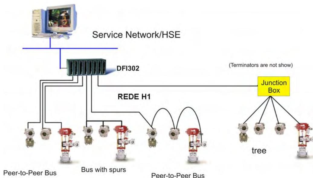
Figure 1.16 – Examples to the Fieldbus Topology
