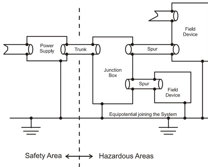
Figure 1.18 – Ideal Combination of Shield and Grounding
