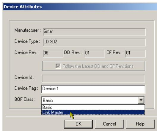
**Figure 3.8 - Configuring the Link Master Device**
