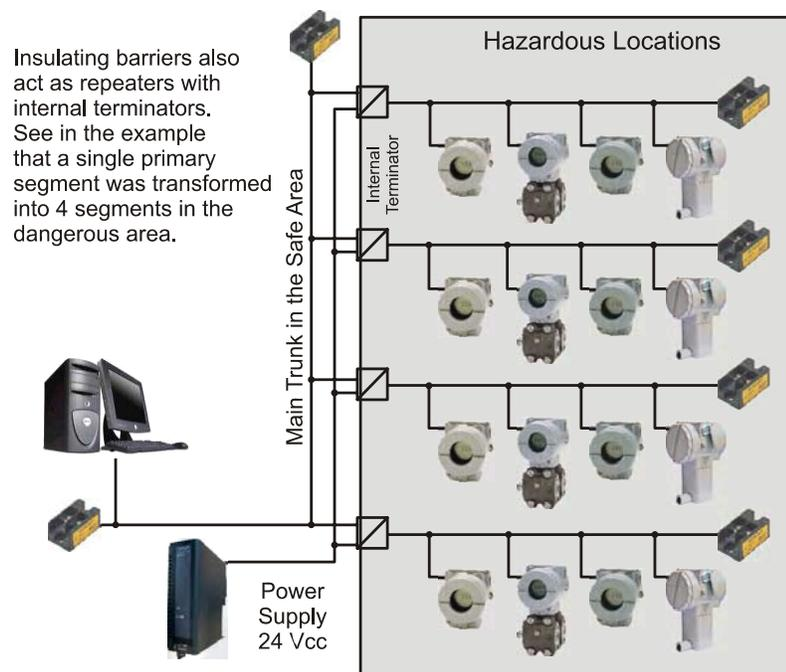
Figure 1.12 - Isolation Provided by the Barrier
