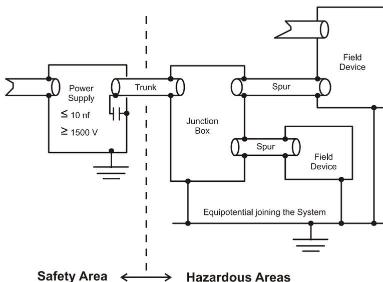
**Figure 1.19 – Capacitive Grounding**
