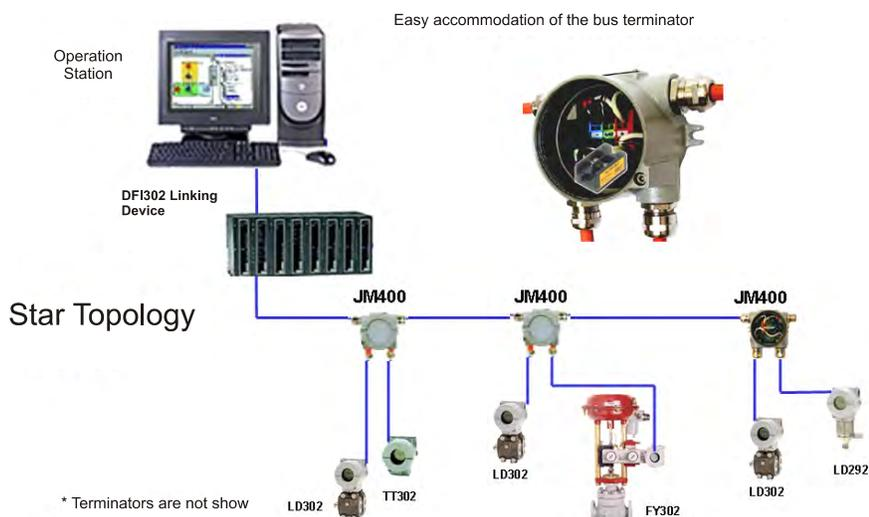
Figure 1.13 - Field Network with Derivation Box
