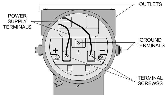
**Figure 1.2 - Wiring Block**
