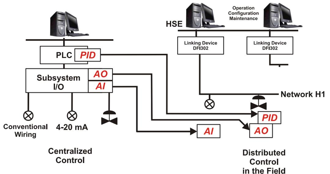
Figure 1.6 - Comparison of Wiring and Distribution of Control over the Network Devices
