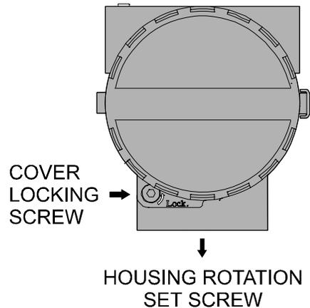
**Figure 1.1 - Housing Adjusting Screw and Cover Lock**
