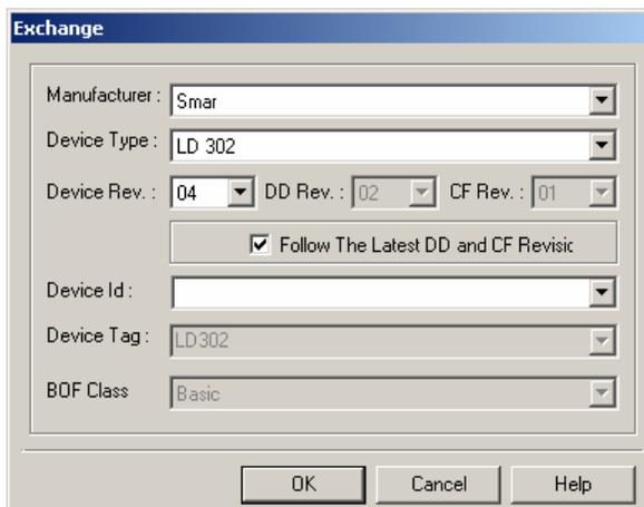
Figure 3.14 - Device Exchange Dialog Box
