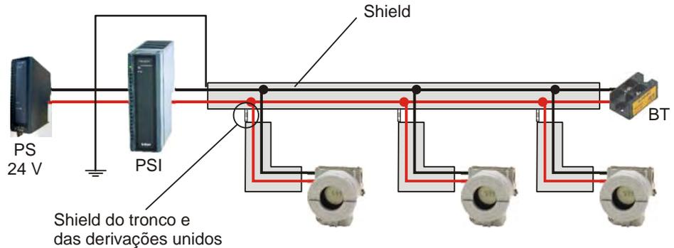
Figure 1.17 – Shield Grounding
