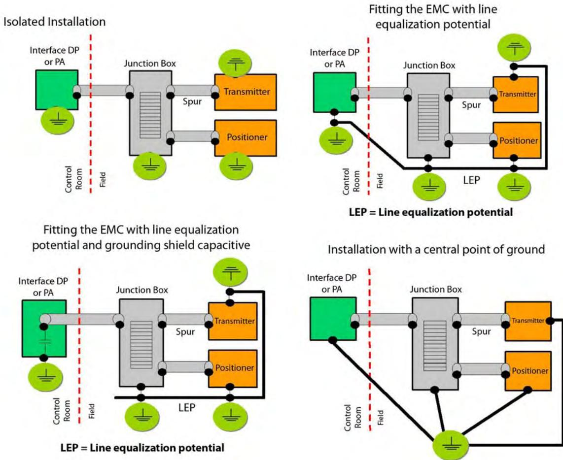
Figure 1.20 – Several Grounding and Shield Ways
