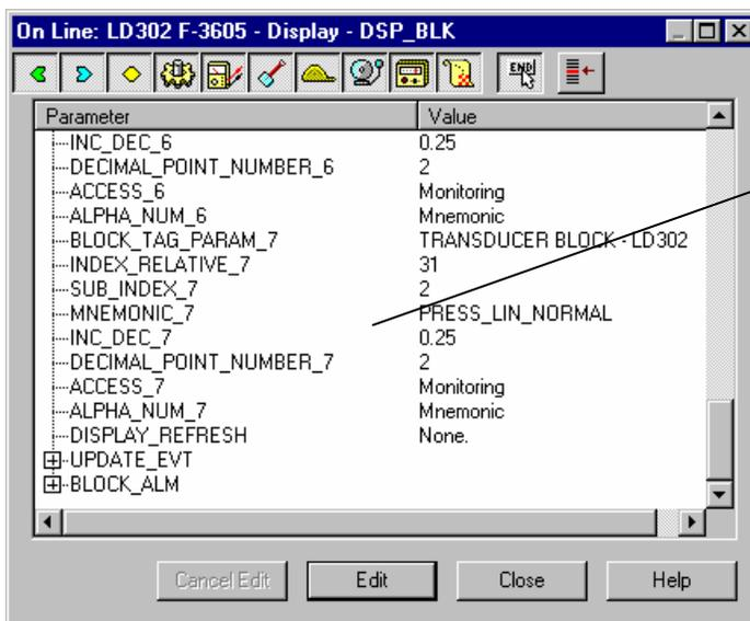
These settings are required to set a parameter on the LCD display.
