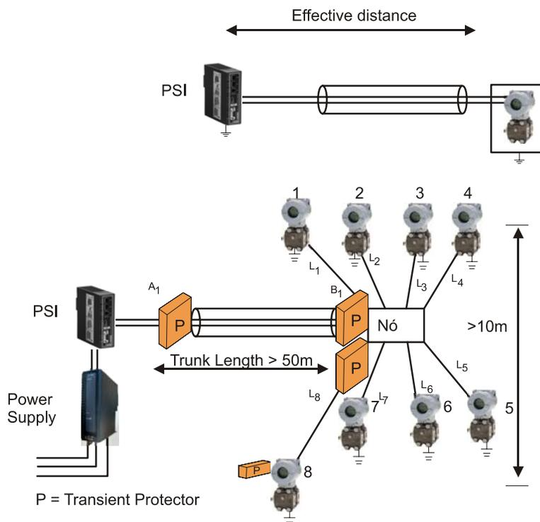
Figure 1.15 – Effective Distance in a Cable Distribution
