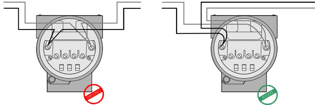
Figure 1.3 – Connecting a device to the Fieldbus network
