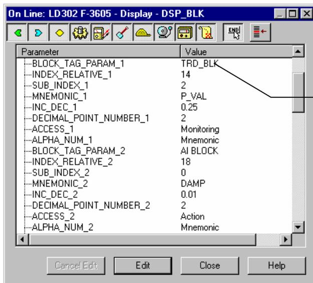
After the first firmware download, the display block will adjust the tags of functional blocks with default values.
