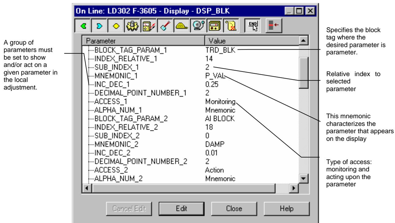
Figure 3.20 – Display of the Transducer – Configuration
