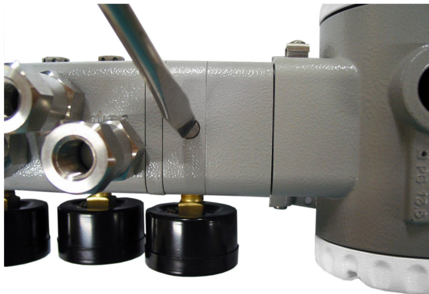
Figure 6.15 – Removing the Restriction Screw
