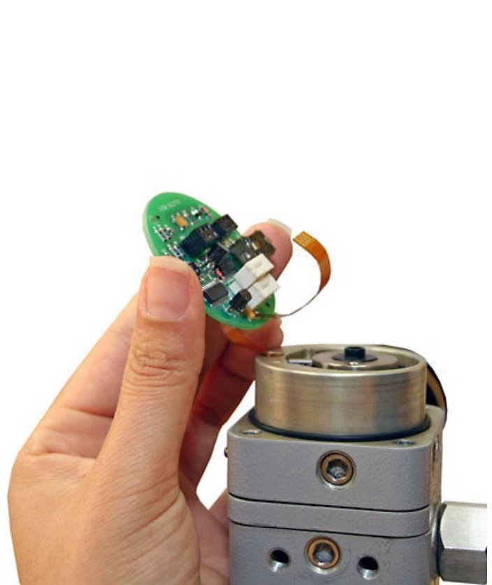
Figure 6.12 - Flat Cable loosened from the connector
