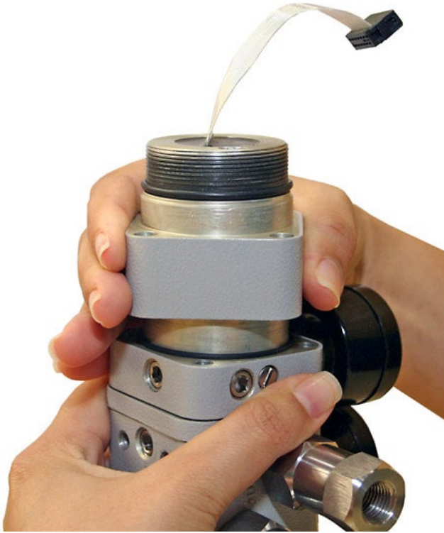
Figure 6.7 – Loosening the Assembled Base Connection Cover
