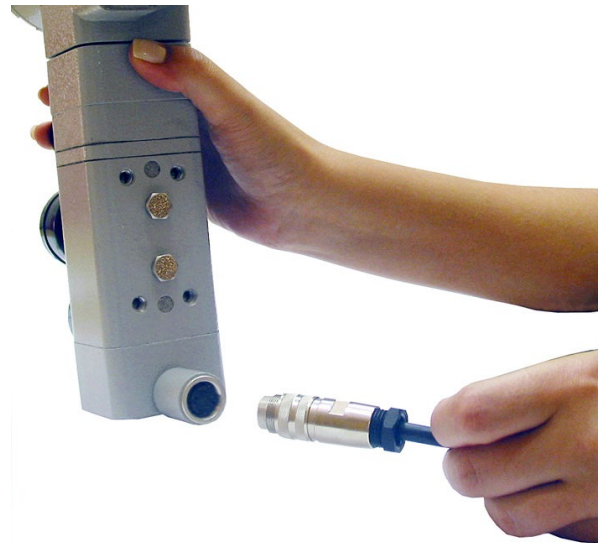
Figure 1.24 – Connecting Cable to the Positioner
