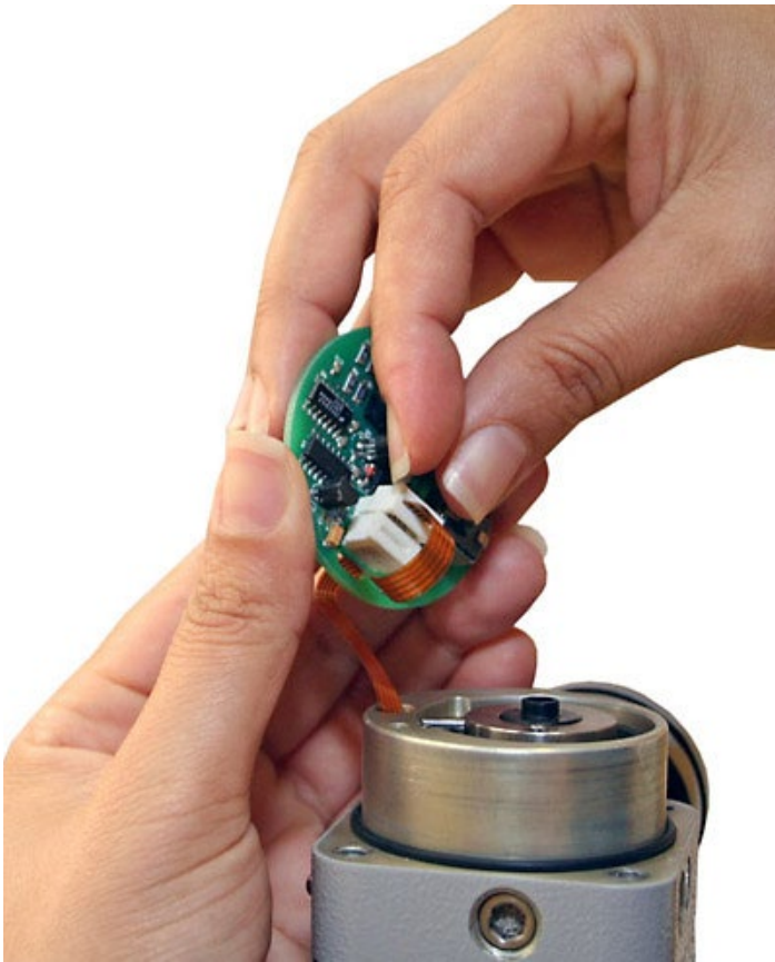
Figure 6.11 – Pulling, with the nail, the lock that fixes the flat cable to the main board
