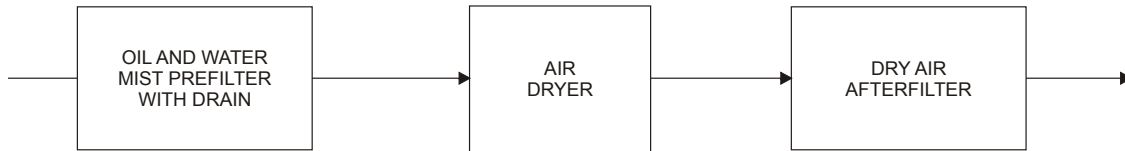
Figure 1.12 - Air Quality Conditioning System
