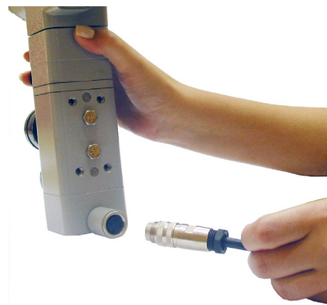
Figure 1.18 - Connecting the Cable to the Positioner
