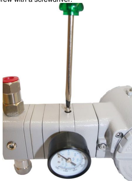
Figure 4.3 – Removing the restriction from the converter
