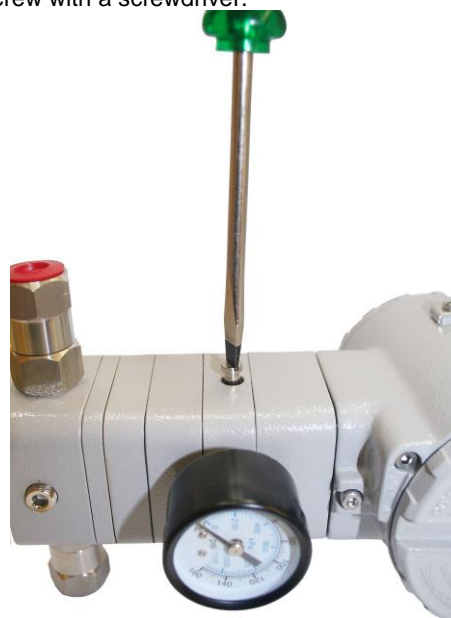
Figure 4.3 – Removing the restriction from the converter
