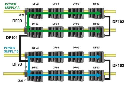
System powered by two power supplies
