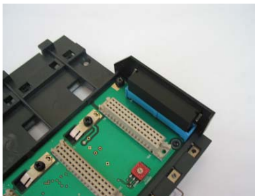
Figure 3.11 - DF2 terminator installed
