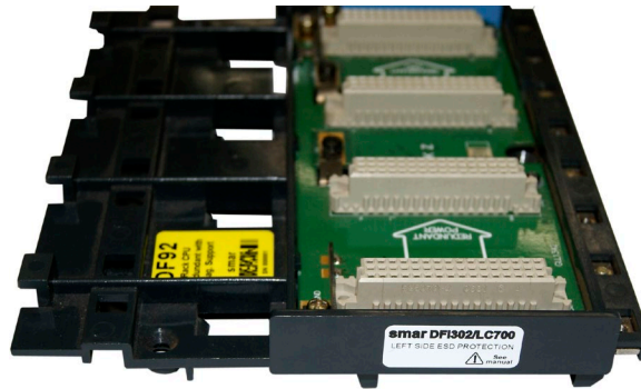
Figure 3. 5 – Left side ESD protection installed on the rack
