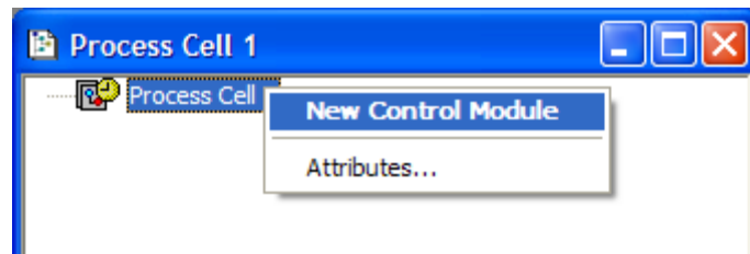
Figure 12.17 – Creating a Control Module
