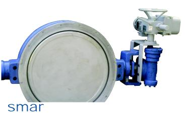
Smar Actuators are available for dampers, gate, slide, diaphragm, globe, butterfly, ball and plug valves. Four torque ranges from 20 to 80 Nm, and rotations from 6 to 48 rpm are available. Higher torque may be obtained by adapting additional gear stages coupled to the output shaft of the actuator.
