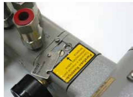
Figure 5.20 - Transducer Serial Number Plate Removed
