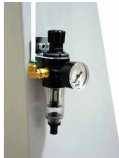
Figure 1.31 – Air Filter Detail
