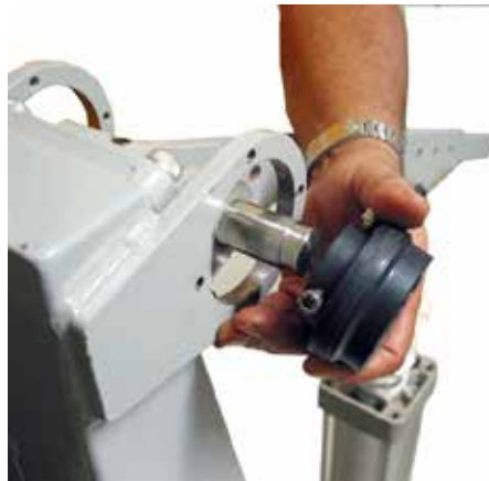
Figure 1.18 - Placing the Magnet
